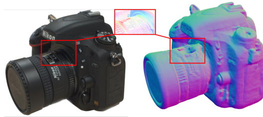
Figure 14: Visualization of distorted mesh resulted by shading.
